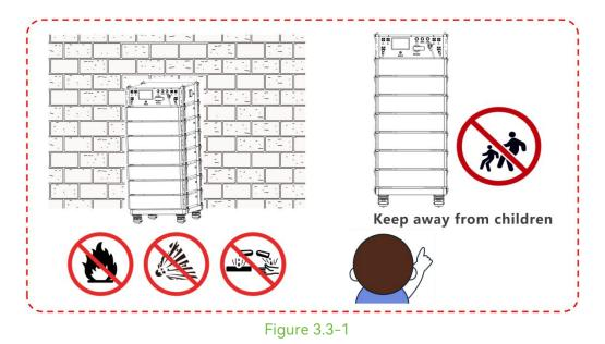
2. Notes on the installation location: Avoid installing near water pipes, cables, etc. inside the wall to prevent damage to the battery . The installation environment should avoid direct sunlight, rain, and snow. It is recommended to install it in a well-ventilated place indoors . If necessary, install an air-cooled air conditioner.
