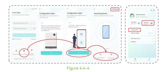
**Note:** Connect by scanning the QR code or inputting the device serial number to correctly configure the battery;
